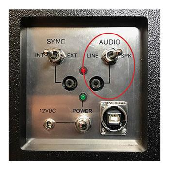
There are two audio switch positions on the module: "Line" and "Speaker".
