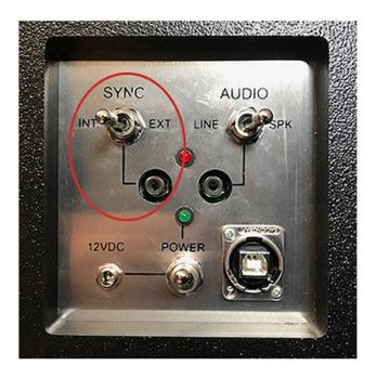
There are two sync switch positions on the module: "Internal" and "External".
