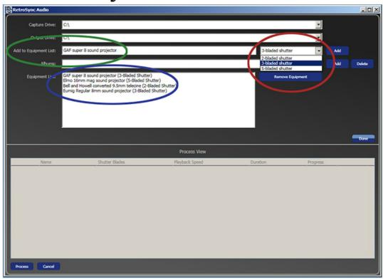
You have a choice of 2, 3 or 5 bladed projectors. The software defaults to 3 shutter blades (most common). Make your selection, write a description of the projector, and click "add". Your projector(s) will appear in the window below. For equipment with once per frame switches or pulse generators, choose "External Sync".
