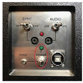
Connect the provided 12 volt DC power supply to the power socket circled above. The AC power cord is standard for North America but can be changed to one appropriate for European standards. When the power switch is in the up (on) position, the green tally light will illuminate.
