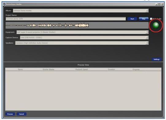
The green icon will pulse on an off if the software is receiving sync pulses correctly. If the icon does not pulse, the software will not record anything. If this happens, check the alignment of the projector and your Capture Device settings.
