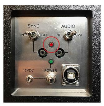
Connect the provided USB cable to the USB port circled above and then connect the other end of the USB cable to your PC running the RetroSync software. Any 64 bit Intel based PC running Windows 7,8 or 10 will work fine. CPU speed is not critical. When the unit is capturing film, the red led circled above will flash if alignment is adequate and the software settings are correct. Do not continue capturing and check alignment and settings if red light is not flashing.
