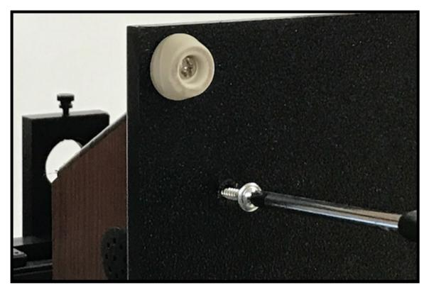
Attach the black plastic bottom to the scanner base and reattach all cords.
