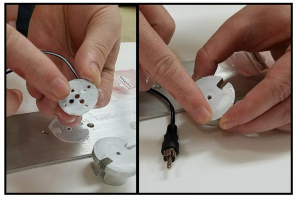
The purpose of the thermal paste is to transfer the heat from the LED down through the LED post to the aluminum plate. So it is impotant to get an even, thick coating of the paste on both pieces. The paste will wash off your finger easily. 5
