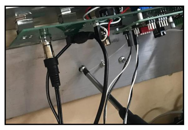
Use a medium Phillips screw driver and remove both retaining screws.
