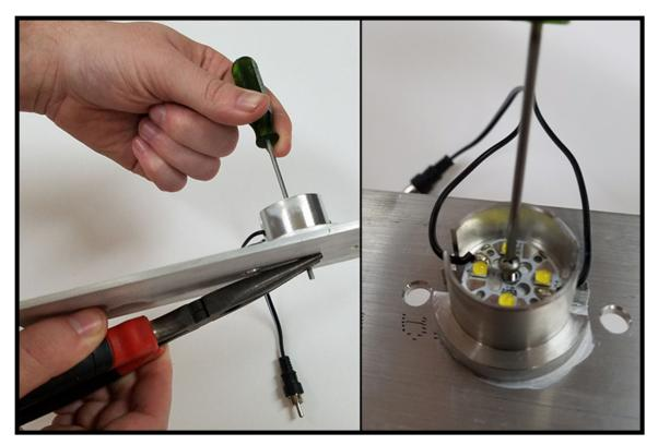
Use a screwdriver and a pair of pliers to tighten the assembly tightly together. If a replacement lock nut is provided, use that in place of the original nut.
