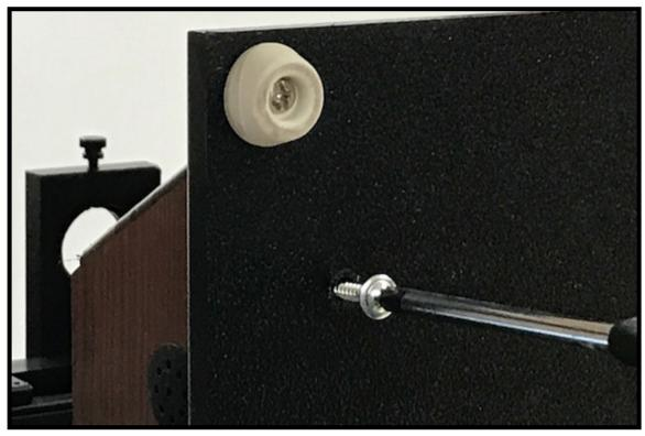
Lay the unit on its back and remove the 4 screws holding the base to the control box. Please note orientation of the rounded front edge of the base.
