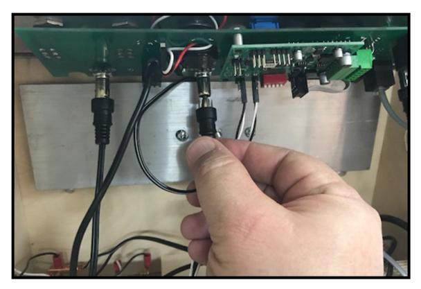
Plug the LED assembly into the electronics.
