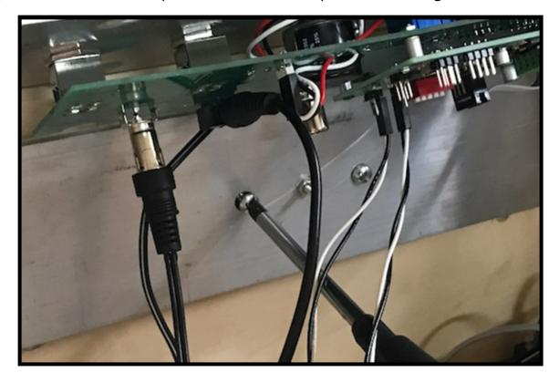
Place the finished assembly back in the scanner and secure using the screws.
