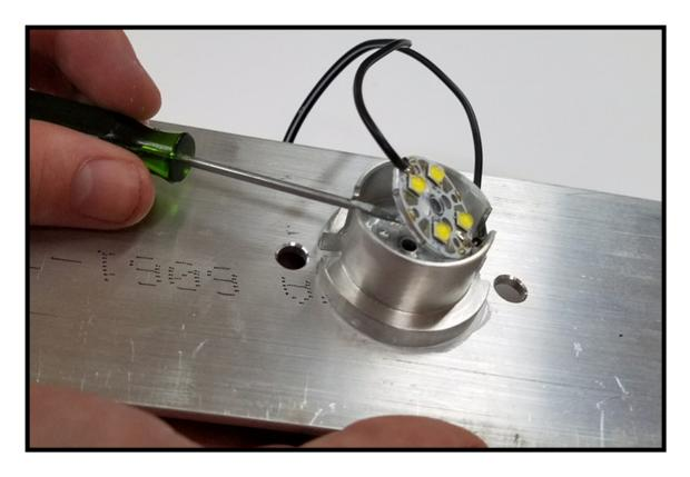
Carefully remove the LED disc and the LED post from the assembly.
