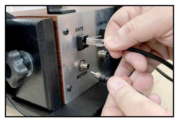
First, remove the camera and any gate that might be on the unit. Then be sure to unplug all cables in the back of the Universal and gently move them aside.
