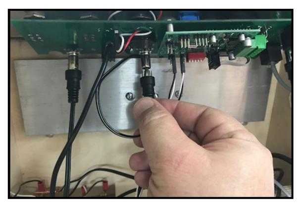
Unplug the connector for the LED assembly.
