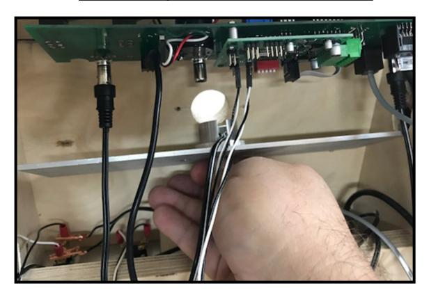
Carefully remove the LED assembly from the base. Avoid accidentally unplugging any of the other cables, if possible.
