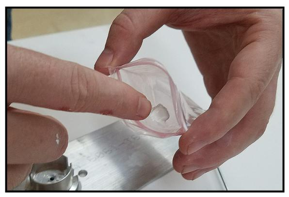
Open the provided bag of thermal paste and, using your finger, apply a thick coating to the back of the LED disc as well as the LED post.
