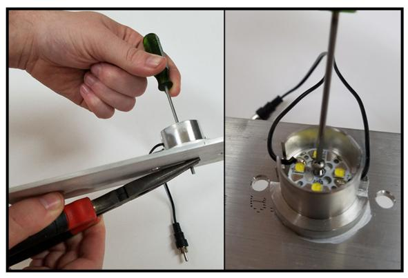
Use a small phillips or flat blade screwdriver and a pair of pliers to remove the center bolt that holds the assembly together.
